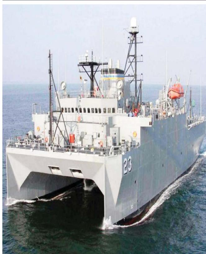
**This March 9, 2009 US Navy photo shows the military Sealift Command ocean surveillance ship USNS Impeccable (T-AGOS-23) one of five ocean surveillance ships that are part of the 25 ships in the Military Sealift Command Special Mission Ships Program. Impeccable directly supports the Navy by using both passive and active low frequency sonar arrays to detect and track undersea threats. — AFP**
